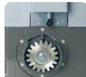
Integrated limit-switch in opening and closing
